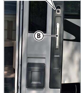
*Fig.5.2 - Opening/closing the entrance door from the inside*
