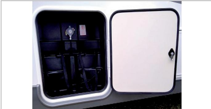
Fig.6.26 - Gas cylinder compartment
