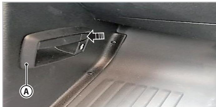
Fig.5.9 - Bonnet opening lever - Type B
