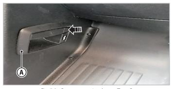
Fig. 5.9 - Bonnet opening lever - Type B
