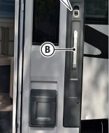
Fig. 5.2 - Opening/closing the entrance door from the inside
