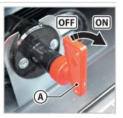
Fig.6.30 - Battery disconnect switch
