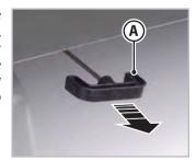
Fig. 6.35 - Grey water drain valve
